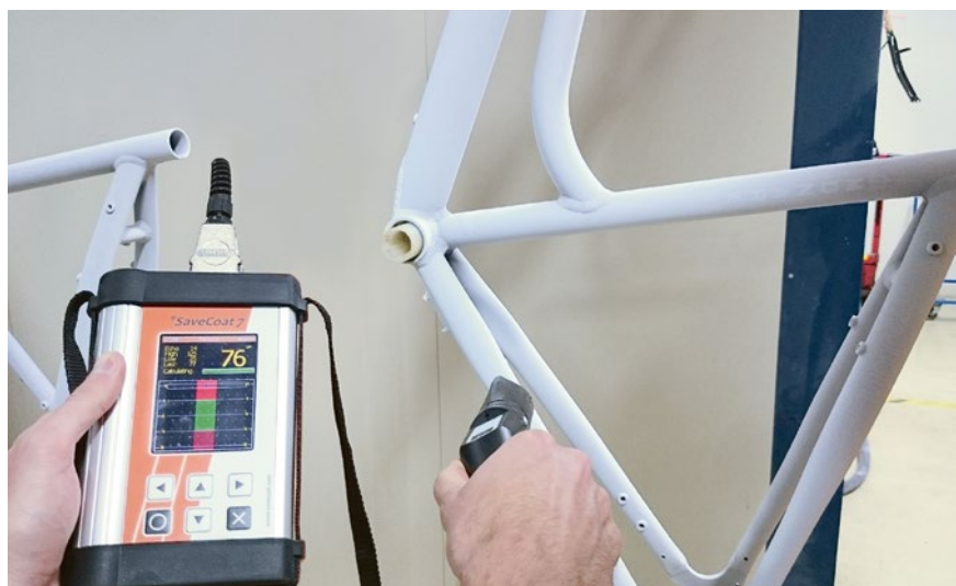
Figure 1 > Hand-held ultrasonic devices can produce reliable measurements even on curved surfaces, such as this cycle frame.
